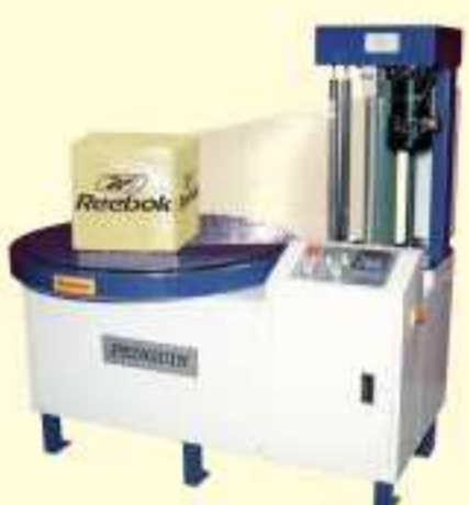
BOX WRAPPER Productivity: 30-75 packs/hour Applications: Apparels, garments, food products, computers, etc., packed in carton boxes
