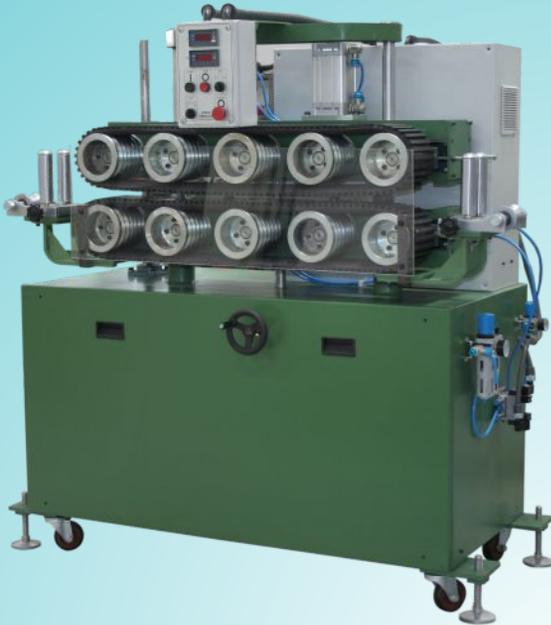
Penguin manufactures caterpillars with modular concepts for utilization in various applications like hose extrusion, hose printing line, braiding line etc.
